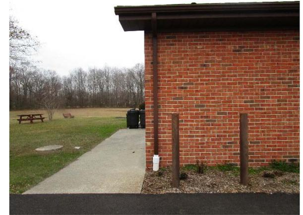
A rain garden can be placed to the north of the building to capture, treat, and infiltrate stormwater runoff and can also provide aesthetic value and create wildlife habitat. A preliminary soil assessment suggests that more soil testing would be required before determining the soil's suitability for green infrastructure.
